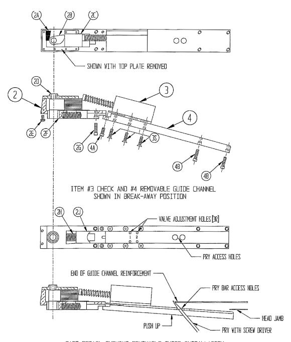
PART DETAIL SHOWING REMOVABLE GUIDE INSTALLATION
