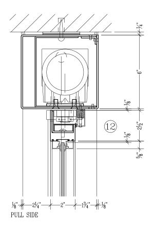
Note: Side load type power operator configurations shown at details 9 & 12 (consult factory for optional bottom load configuration if required for recessed header applications)
